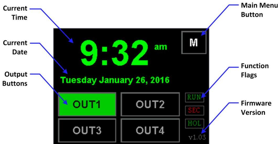
The main screen of the controller indicates the current time and date, the state of the four outputs, function flags that indicate whether the controller is running the output schedules, has security enabled for accessing the controller schedules and configuration, and whether holidays are enabled and active.
